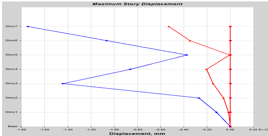
Figure 9: Story displacement of conventional concrete in zone III in X- direction & Y- direction
